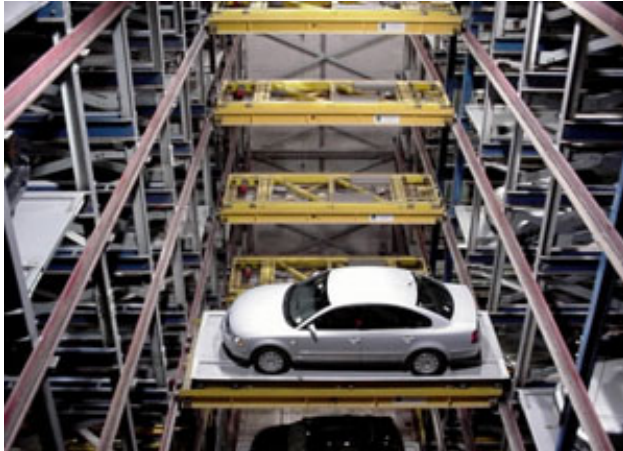
Photo by: Parking Systems, Inc. An automated system lifts cars into place in this parking garage in Hoboken, NJ.
